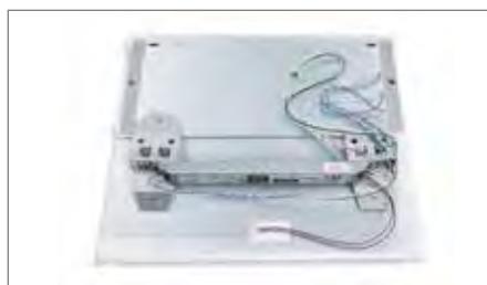
Step 1: EvokitSR is shipped with a plate covering the sensor hole. There are two wires secured to the back of the plate.
