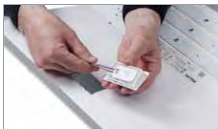
Step 4: Take these two wires and insert them into the sensor. They are not polarity sensitive.
